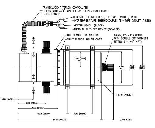
MODEL NUMBER: TIHAV-(10-30kw)-Vxxx-FCXX-Dxx INLET/OUTLET: FC100 = 1.0" FLARETEK FITTINGS FC75 = 3/4" FLARETEK FITTINGS FC50 = 1/2" FLARETEK FITTINGS DRAIN FITTING: FC75 = 3/4" FLARETEK FITTING FC50 = 1/2" FLARETEK FITTING
